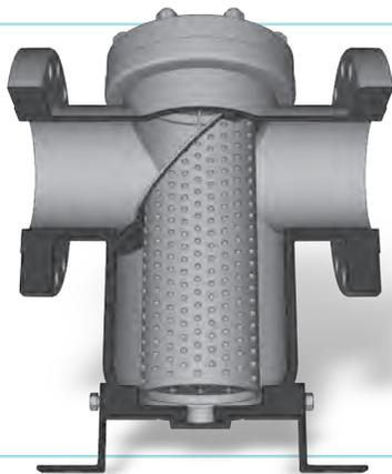
**BASKET STRAINERS** are used commonly in horizontal applications where cleaning will be less frequent. Because of their larger bodies, they typically provide more open area for debris collection than Y-strainers. The straining element (a.k.a the "basket") for a basket strainer has a handle for easy removal and secure placement within the strainer's body. The basket can have a slanted top design (as shown to the left) or a straight top design.
